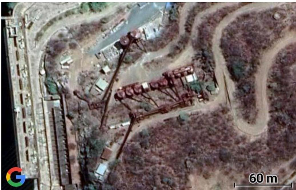
**Figure 5-47 - HCB- traces of infrastructures from the time of the construction of the dam**
